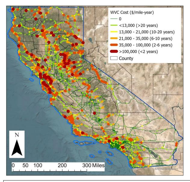
**Figure 9.** Annual cost of WVC per mile. The time in parentheses in the legend indicate how many years of reduced WVC on a highway segment would have the equivalent cost of fencing along that segment. For example, "<2 years" indicates that the cost of fencing that segment is the same or less than the fiscal benefit of reduced WVC for <2 years.
