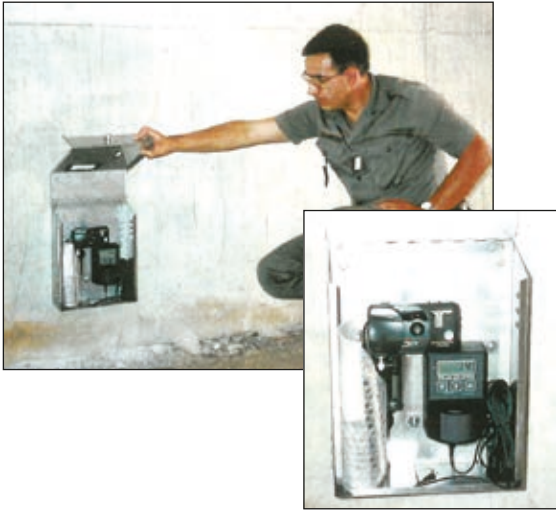
Photos n°1: Silver process camera trap used in the 1990s. (© VINCI Autoroutes, OGE)
